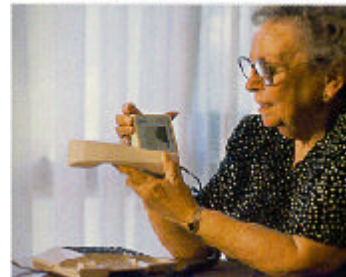
Left. Transmit ECG recordings over telephone lines to a receiving station for storage or interpretation.
