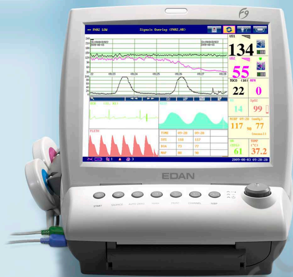
12 inches high-resolution color LCD, folding up, touch-screen (optional)
