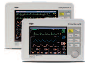
Infinity Gamma X XL Portable bedside/transport monitor with 10.4" (264 mm) color display; 5 channels (6 optional)
