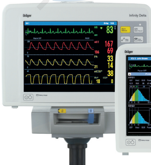
Infinity Delta: 10.4" (264 mm) screen; 12.7 lbs (5.8 kg) Infinity Delta XL: 12.2" (310 mm) screen; 13.6 lbs (6.2 kg)
