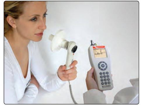
Display: Black and white LCD display (320x240 pixels) with realtime monitoring of test performance, plus encouragement features for children and non-compliant patients
